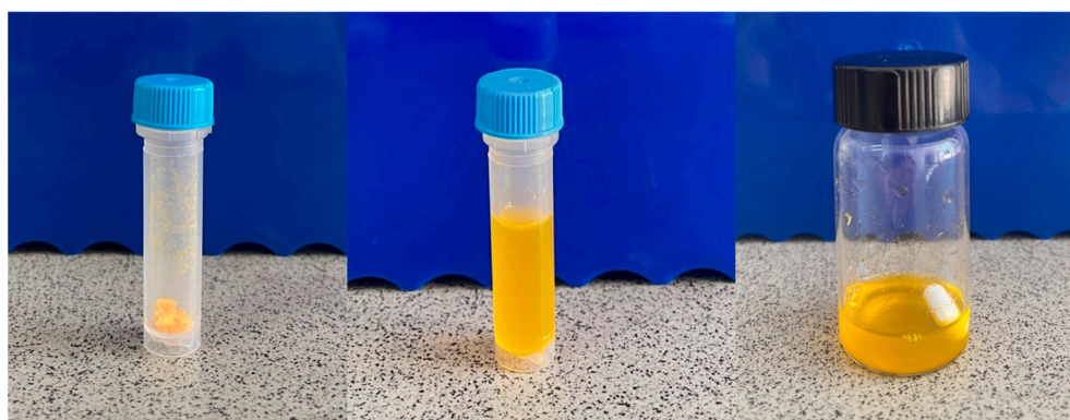
Figure 3. Lyophilized BSA-FITC/DMPG complex formed via hydrophobic ion pairing ( left ). ST-SNEDDS-BSA-FITC/DMPG, i.e., transparent oily solution consisting of a mixture of Labrafil M 1944 CS, Kolliphor HS15, Squalene and \alpha -Tocopherol, where the BSA-FITC/DMPG complex has been dissolved with the aid of vortex and sonication at a 40% amplitude for 2 min in an ice bath with a microtip sonicator ( middle ). ST-SNEDDS-BSA-FITC/DMPG oil-in-water (o/w) nanoemulsion spontaneously formed by the dropwise addition of PBS to the oily solution ST-SNEDDS-BSA-FITC/DMPG under magnetic stirring ( right ).
